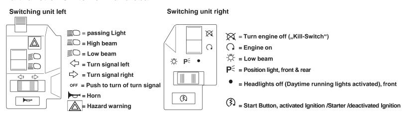
To flash in a desired direction, you must briefly press the switch in the desired direction. To stop the flashing, press the center of the switch forward.
