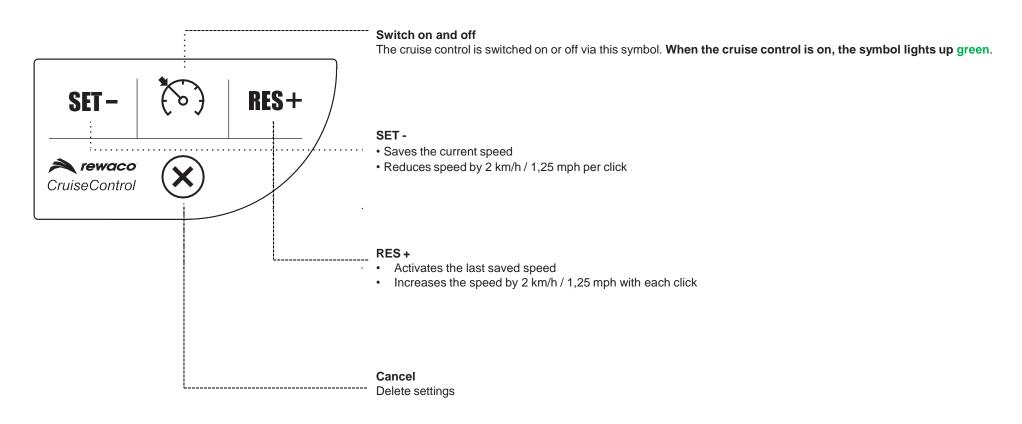
If you brake while the cruise control is activated, the automatic cruise control is interrupted and can be reactivated by pressing the "RES+" key.
